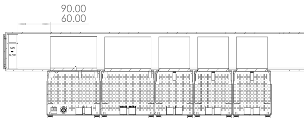
Figure 4-6: AMD5x system fan clearance to first PIU heatsink
