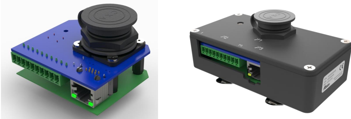
Figure 4-3 Pendant Patch Board Mk2 and Mk2 Enclosure
