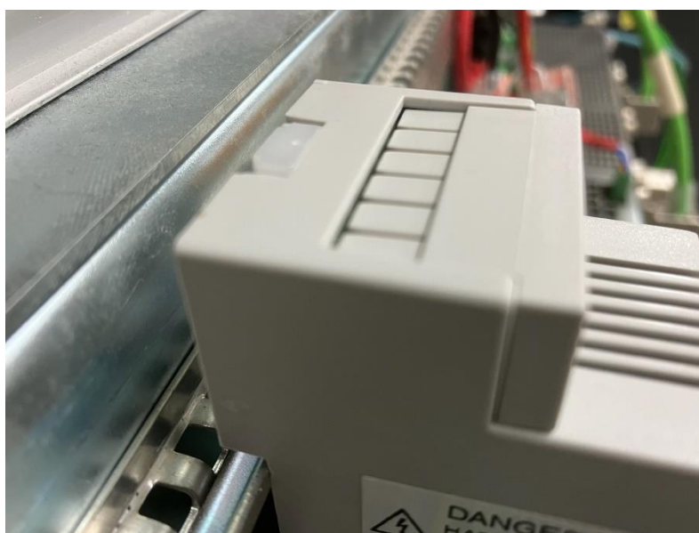
Figure 6-12 Ensure the White Clip is Fully Inserted
