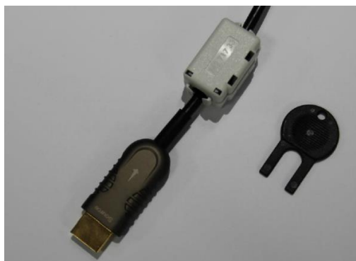
Figure 9 - Ferrite core on hybrid optic fibre cable
