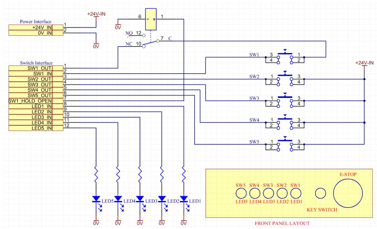
Figure 10-2 Touchpad Switch Interface Wiring Diagram
