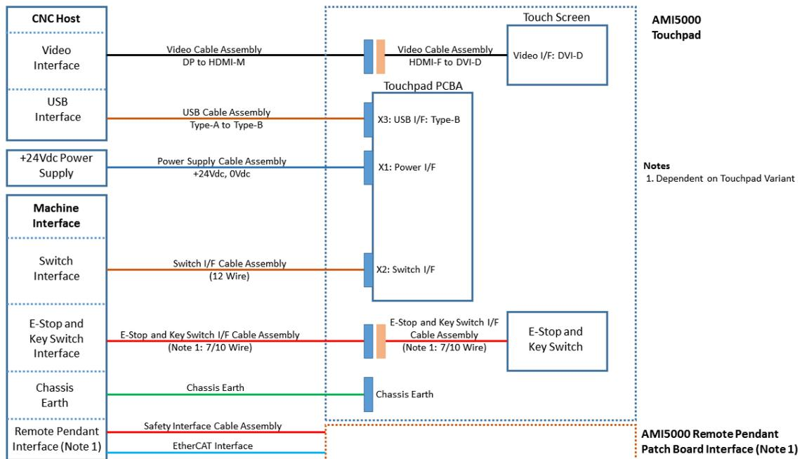
Figure 5-7 Touchpad Wiring Diagram
