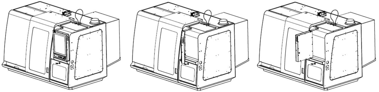
**Figure 4-1 Typical installation of the AMI5000 Touchpad on a Customer Machine (also showing the range of rotation)**
