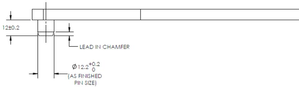
Figure 13-3 Upper Pivot Bracket Dimensions: Pivot Variant
