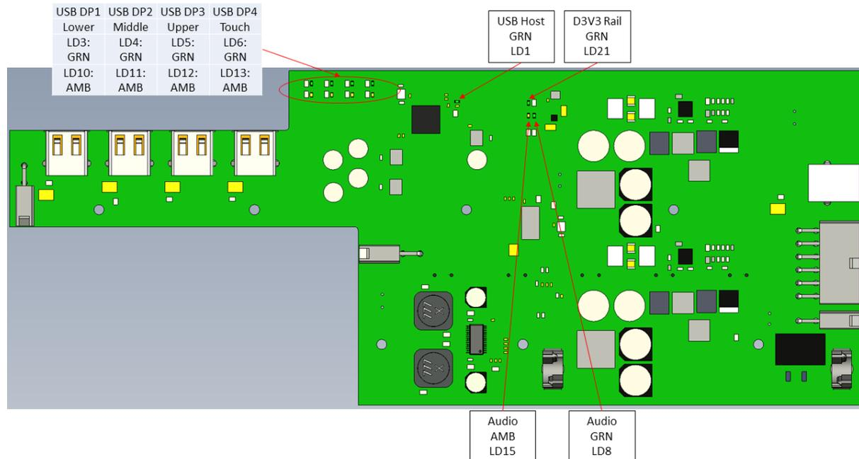
Figure 11-1 Touchpad Board Diagnostic LED Indicators
