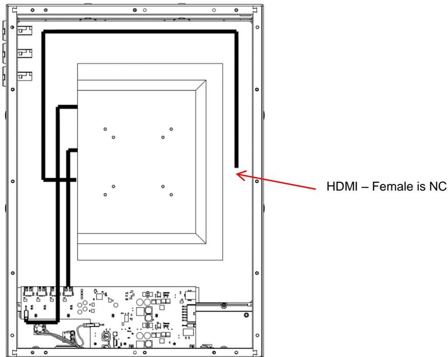
Figure 5-5 Digital Video Interface Connector on the Touchpad (viewed from the rear of the unit)
