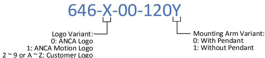
Figure 3-3 Mounting Arm Variant Product Number Breakdown
