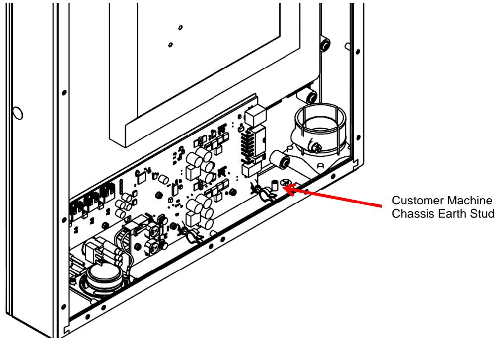
Figure 5-6 Customer Machine Chassis Earth Stud (viewed from the rear of the unit)
