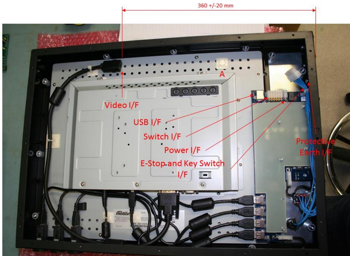
**Figure 4-3 Mounting Arm Variant: Internal Interface Connector Reference**
