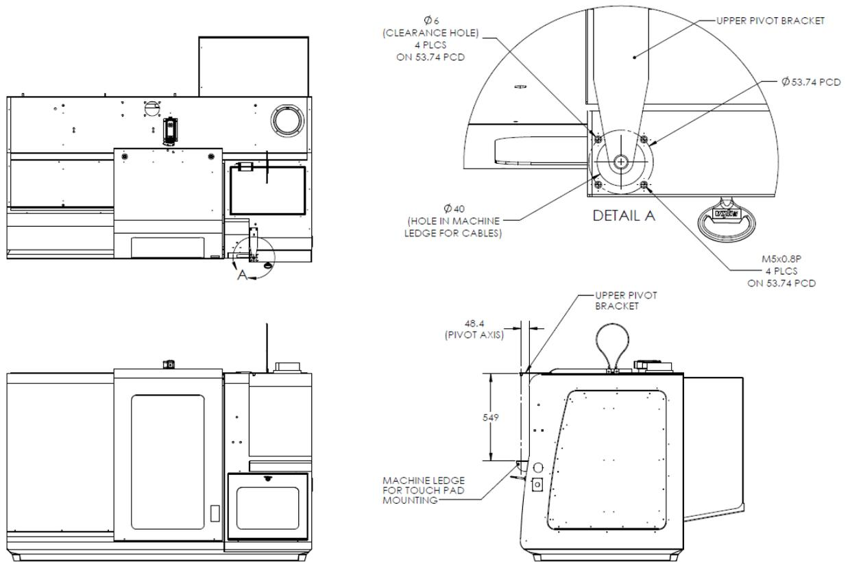
Figure 13-2 Fitment Dimensions for Typical Machine: Pivot Variant
