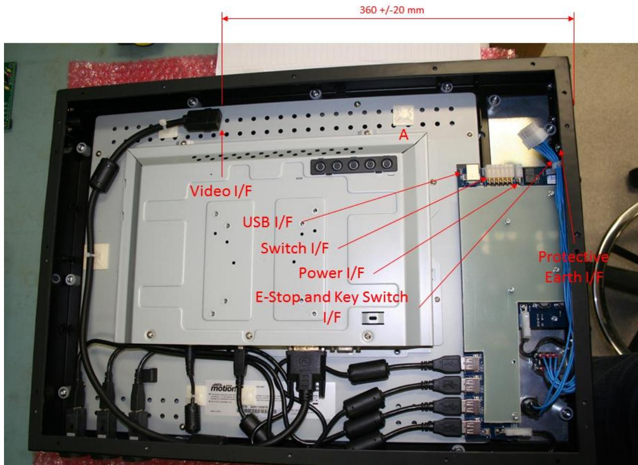
Figure 4-1 Pivot Variant: Internal Interface Connector Reference
