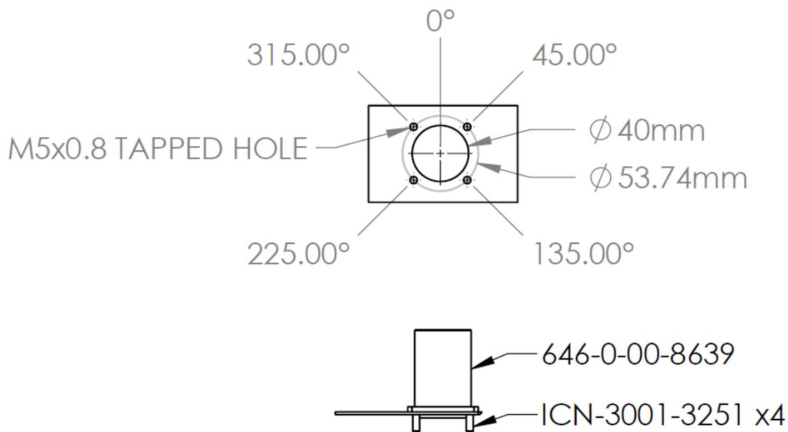
Figure 13-4 Lower Pivot Mounting Details: Pivot Variant
