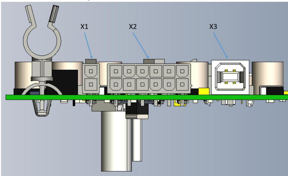
Figure 5-1 Interface Connectors on the Touchpad Board
