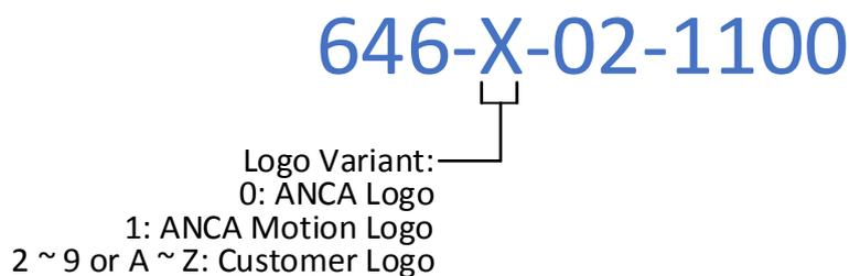
Figure 3-2 Pivot Variant Product Number Breakdown
