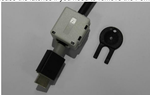
Figure 7 - Ferrite core on copper HDMI cable
